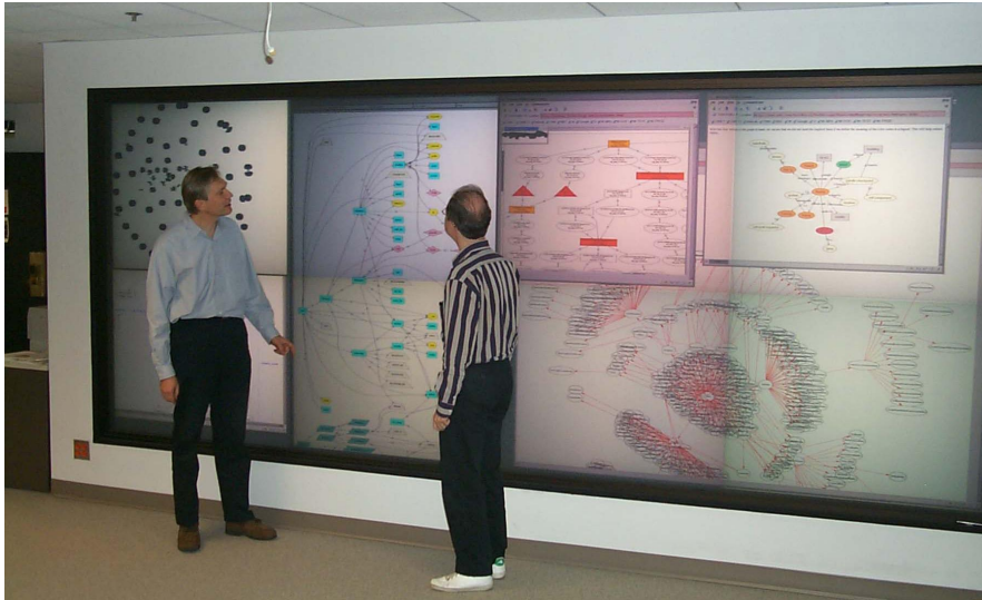
Fig. 4. Information visualization with graph drawings on a 10 megapixel display wall. The displays include maps of virtual private networks, a section of the public Internet, and software engineering diagrams. The visualizations are an important complement to conventional text and statistical displays for exploring large, semi-structured information sets
